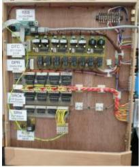
switched mounted on the point motors, these provise the point position feedback. The connector with the grey wires would normally be connected directly to the module, the breakout arrangement here was to allow the point position to be fed to a separate demonstration, as was the ribbon cable connected to the DTC. Lastly on this stack is a RSM (Remote Stack Master), not used here.
