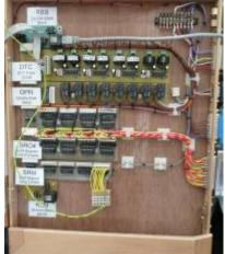
switched mounted on the point motors, these provise the point position feedback. The connector with the grey wires would normally be connected directly to the module, the breakout arrangement here was to allow the point position to be fed to a separate demonstration, as was the ribbon cable connected to the DTC. Lastly on this stack is a RSM (Remote Stack Master), not used here.
