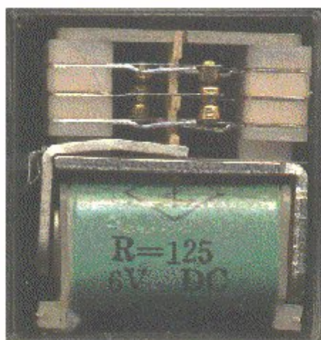
Relay showing coil and switch contacts
