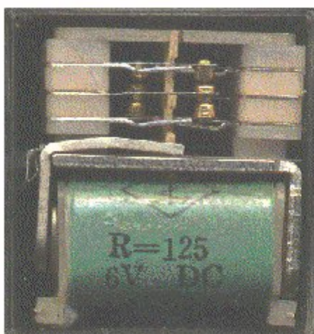
Relay showing coil and switch contacts
