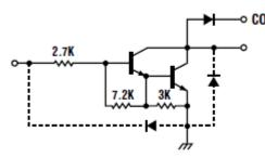
In electronics, the Darlington transistor is a semiconductor device which combines two bipolar transistors in tandem (often called a "Darlington pair") in a single device so that the current amplified by the first is amplified further by the
