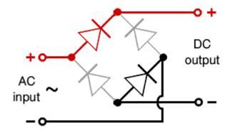
The diagram shows the operation of a bridge rectifier as it converts AC to DC. Notice how alternate pairs of diodes conduct.
