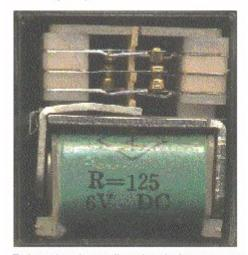
Relay showing coil and switch contacts
