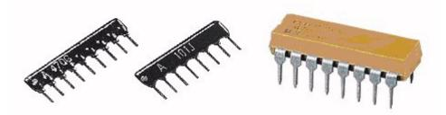
"Resnets" come in 3 basic package types. Pin at one end is common to all (odd number of pins). Individual resistors in single line, pair of pins for each resistor. Individual resistors in DIL, resistors connect to pins on opposite sides of package.
