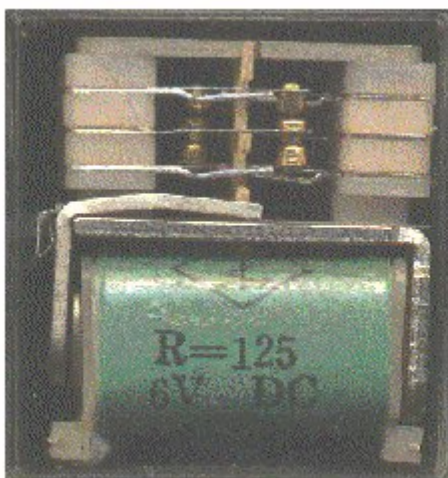
Relay showing coil and switch contacts
