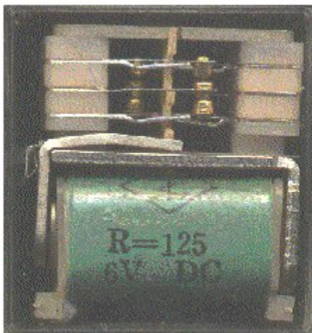
Relay showing coil and switch contacts
