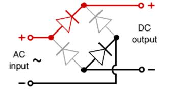
The diagram shows the operation of a bridge rectifier as it converts AC to DC. Notice how alternate pairs of diodes conduct.
