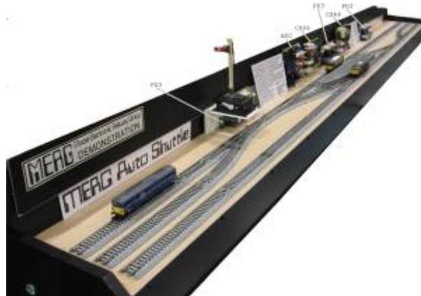
The shuttle module or ATC (Automatic Train Controller) MERG Kit 46, comes preprogrammed with a number of different configurations, selectable using an on board 4 way DIL switch. The track on this [demonstration](#) board is a symmetrical arrangement that allows all of these configurations and the module cycles through these.
