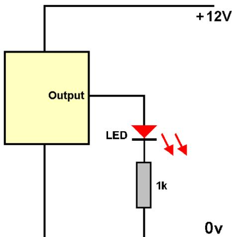
This illustration shows the LED being wired to 0V. In this case, the LED will illuminate when the module's output pin goes high. When the output is low, there is no voltage difference across the LED and it will not illuminate.
