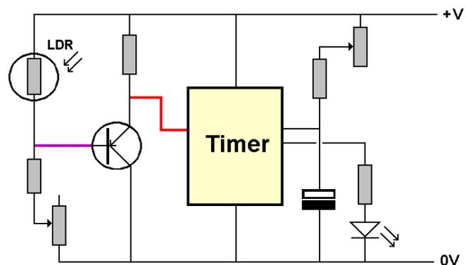
At a certain input voltage level, the transistor's output level will change from high to low. This change is connected to the timer's input – the red line shows the digital interface. The variable resistor determines the voltage fed to the transistor and is used to set the level at which the module switches the LED on and off.
