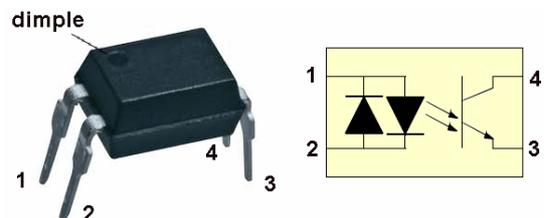
Many optocouplers have a single LED inside its case, but the KB814 has two that are wired opposite to each other. This allows this particular optocoupler to work with an AC input if required.
